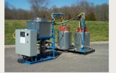
Unit for drying solids (IX resins, sludges, concentrates)
